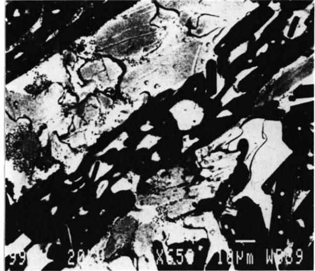
Fig. 2. Electron microscopy image of cuprate decay and beginning formation of 2212 phase.
