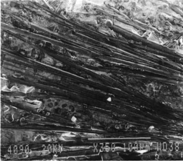
Fig. 1. Electron microscopy image of needle-like crystals of Sr and Ca cuprates in the coating on an Ag wire.
